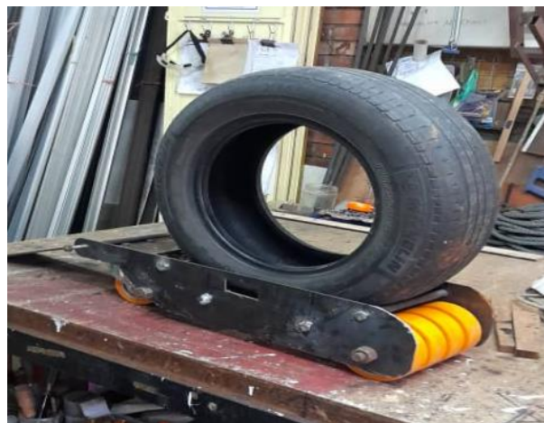
Figure 3 : The position of the tyre inside the Car Skates
