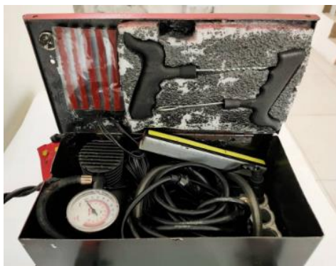
Figure 2: Electric Air Pump, Lamp, Socket Holder and Tubeless Repair Kit
