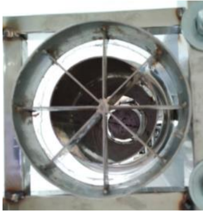
Figure 6: Stainless Steel Cutting Blade
