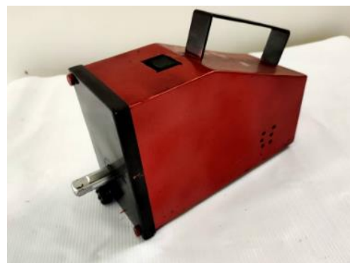
Figure 3: Electric Tyre Wrench
